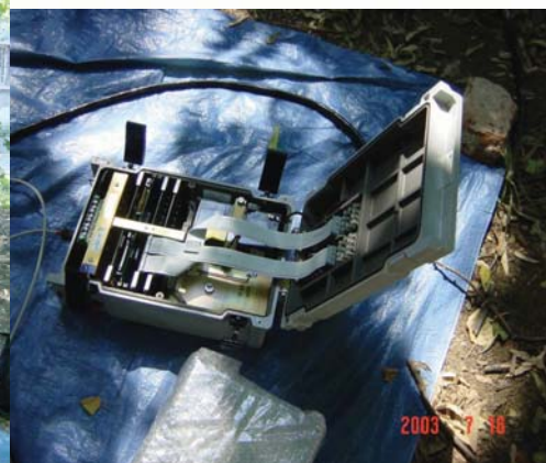
Kinematics K2 station with Episensor & FBA23-DH
