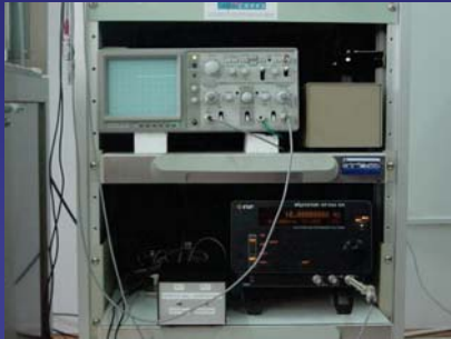
Production of the excitation signal (the -wave synthesizer) and Signal reception (high-resolution oscilloscope)
