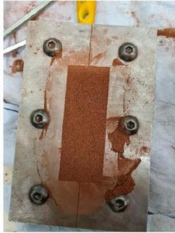
Figure 8 MMS-2 simulants being placed in a rigid mould.
