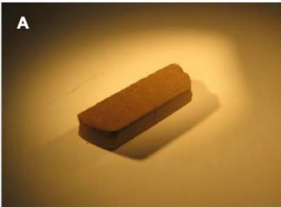
Figure 1. (A) A photo of solid Mars-1a beam quasi-statically compacted with rigid boundary condition. The curved ends show the boundaries of the steel mold. The width of the sample is ~1 cm. (B) Flexural strength of compacted Mars-1a as a function of the initial average particle size. The average particle sizes are computed as the nominal midpoint for each fractioned sieve size, i.e. the arithmetic mean of the bin sizes. The three series represent the three lateral boundary conditions (names in bold) with the maximum compression pressure (in MPa) inside parentheses.
