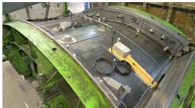
(a) Installation of fibre optic cables inside the casting mould
