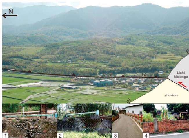
Figure 2. View of the fast creeping Chihshang fault (black line) that bounds Longitudinal Valley and Coastal Range in eastern Taiwan. With 2–3 cm/yr surface slip rate, this is the most rapidly creeping continental reverse fault in the world. The east dipping thrust fault separates by Lichi Mélange in the hanging wall and young river deposits in the foot wall. Fault creep damage of utility pipes (1 and 2), a road (3), and a brick wall (4) along the Chihshang fault in eastern Taiwan. Surface slip on the Chihshang fault is monitored with creepmeters [Lee et al., 2003] (1 and 2). Credit: Hao-Tsu Chu and Chung-Hsiang Mu.
