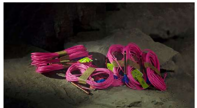
EZshot LP shock tube initiated electronic detonator
