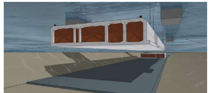
A tunnel element during immersion: cables, winches and advanced measuring equipment guide the element to its exact position.
