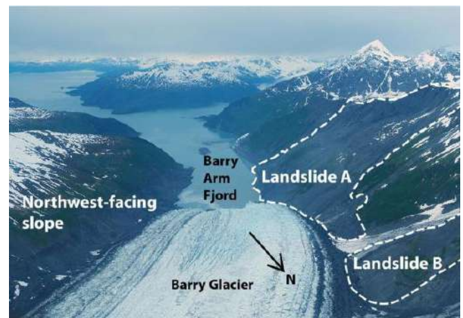
Subaerial landslides could generate tsunamis if they rapidly failed into Barry Arm Fjord in southern Alaska.
