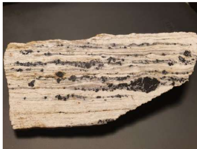
Mylonitic metagranite from the Sierra Nevada, Spain. The original minerals constituting the metagranite (grey = quartz; white: feldspar; black: tourmaline) were deformed and stretched. Tourmaline is stronger than quartz and feldspar and shows brittle behavior even in this mylonitic sample.
