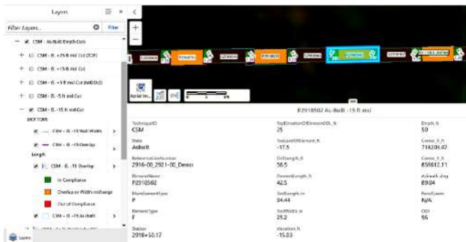
Figure 2. Planimetric GIS web viewer showing the position and overlap of cutter soil mixer panels at a specific depth
