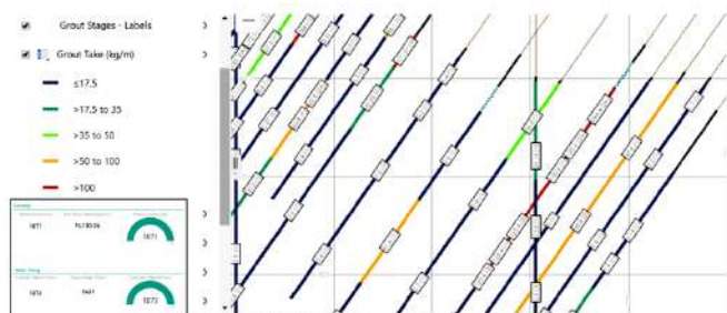
Figure 4. Profile GIS web viewer showing grout stage data and production status
