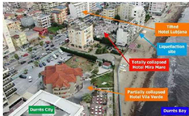
Figure 3. The liquefaction site in the southern part of Durrës was close to three hotels that experienced extensive structural damage: the totally collapsed Mira Mare Hotel, the partially collapsed Vila Verde hotel, and the Lubjana hotel (drone source: Lekkas et al., 2019). 6
