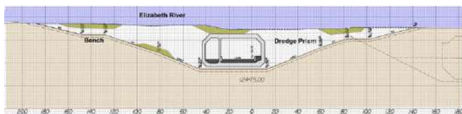
Figure 1. Dredge slope geometry and immersed tube element.
