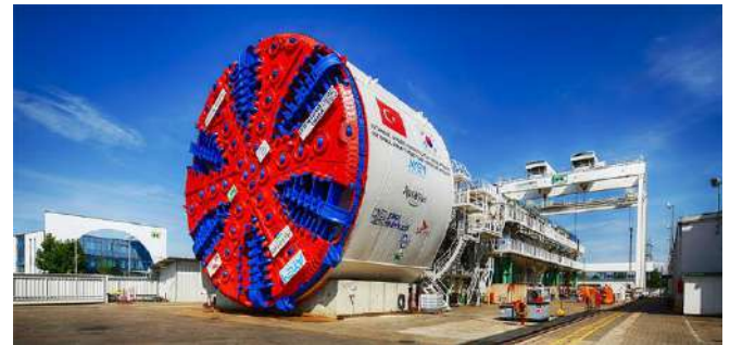
Figure 4. The Eurasia Tunnel TBM, designed for 13-bar hydrostatic pressure cross section.
