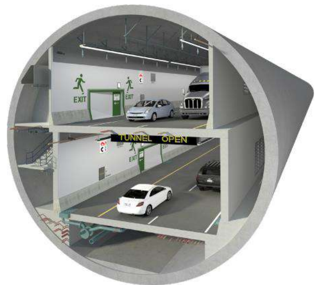
Figure 2. SR 99 tunnel section showing traffic lanes, emergency exits, exhaust air plenums, and utility pathway below the roadway.
