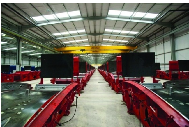
Lines of moulds at the Old Oak Common tunnel lining works
