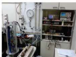
Resonant column device - Drinech type: longitudinal and torsion oscillation
