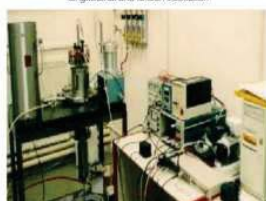
Resonant column and torsion shear device - Hardin type
